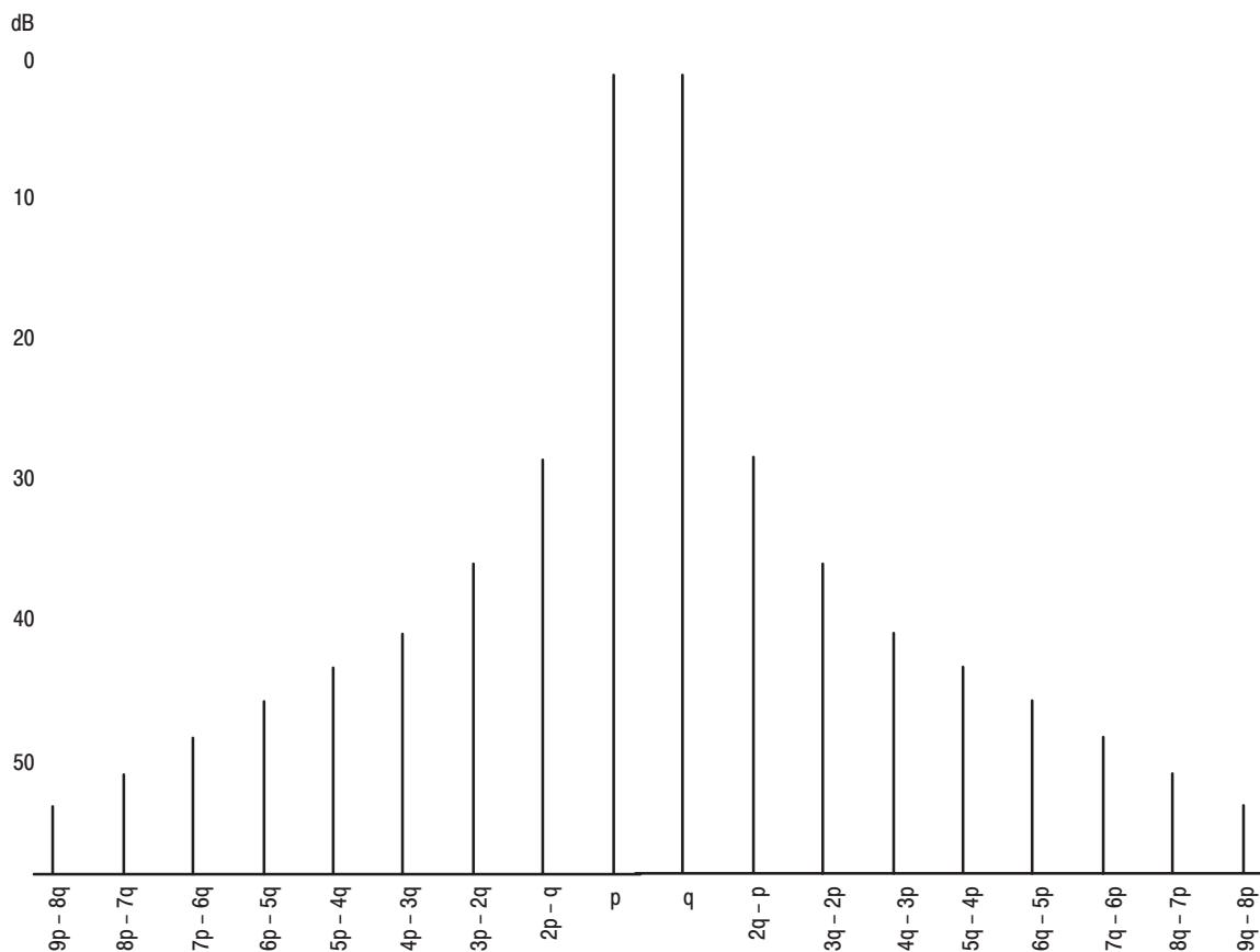
Figure 3. Typical Distribution of Distortion Product Amplitudes Compared to the
