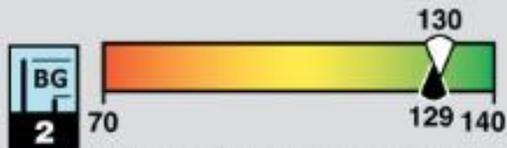
2 kHz Blocking Gain Compression (dB)
