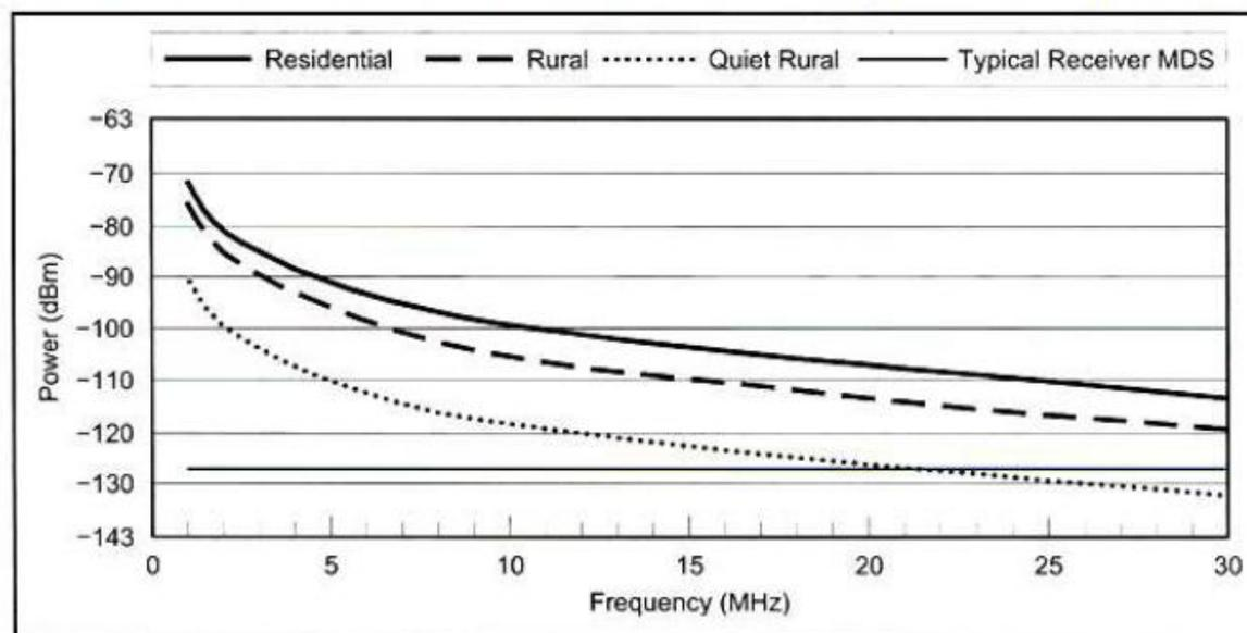
Typical noise levels versus frequency for various environments.
