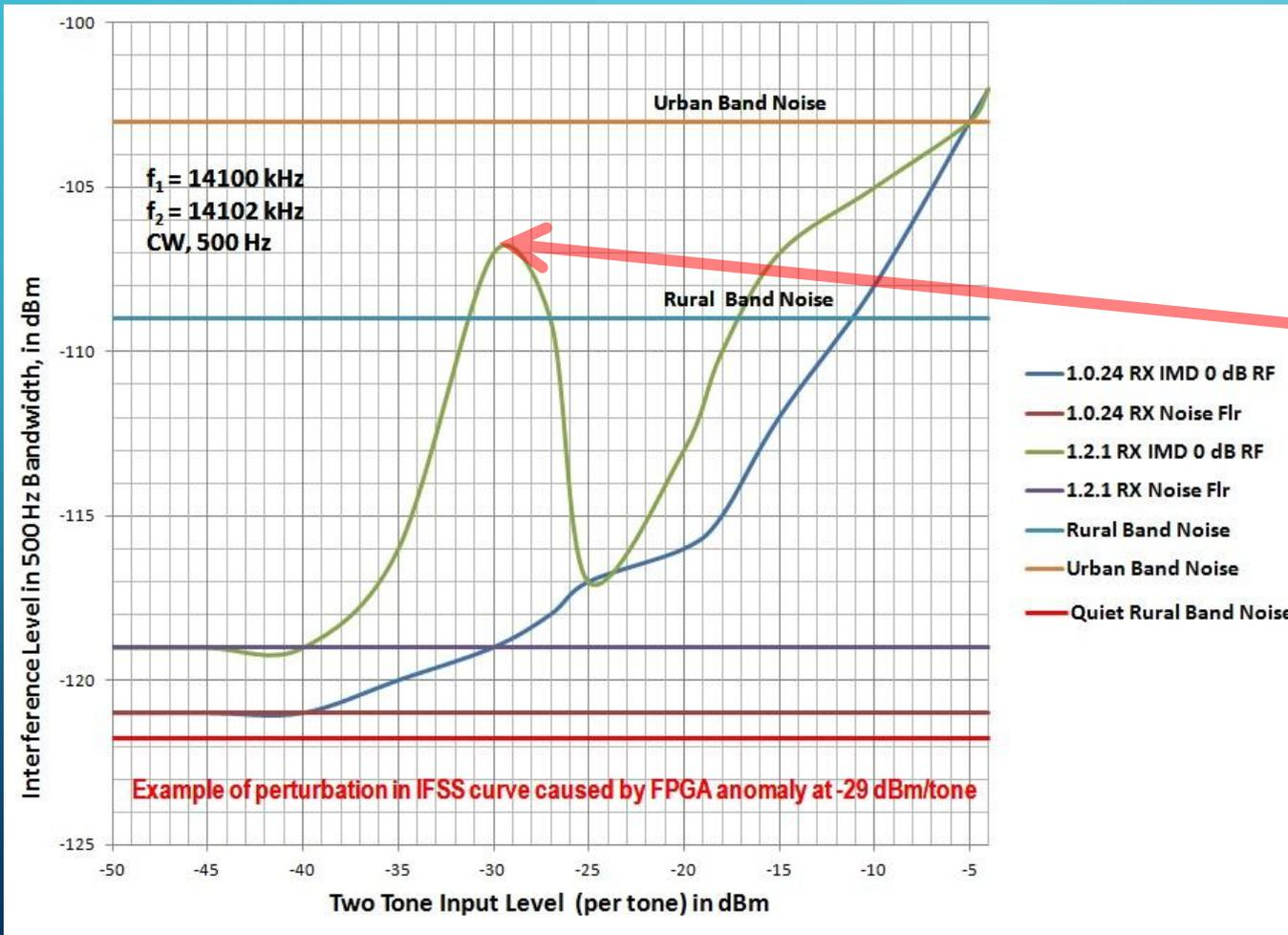
Note IMD amplitude spike at -29 dBm/ton input level, due to an FPGA processing anomaly.
