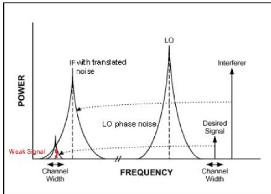
Strong interferer mixes with LO phase noise to “throw” noise into IF channel. If the interferer consists of wideband noise, the IF channel will be filled up with noise. A typical synthesized LO divides its VCO down to cover lower frequencies. Thus, its phase noise will be worst at the top end of its tuning range than at the bottom end.
