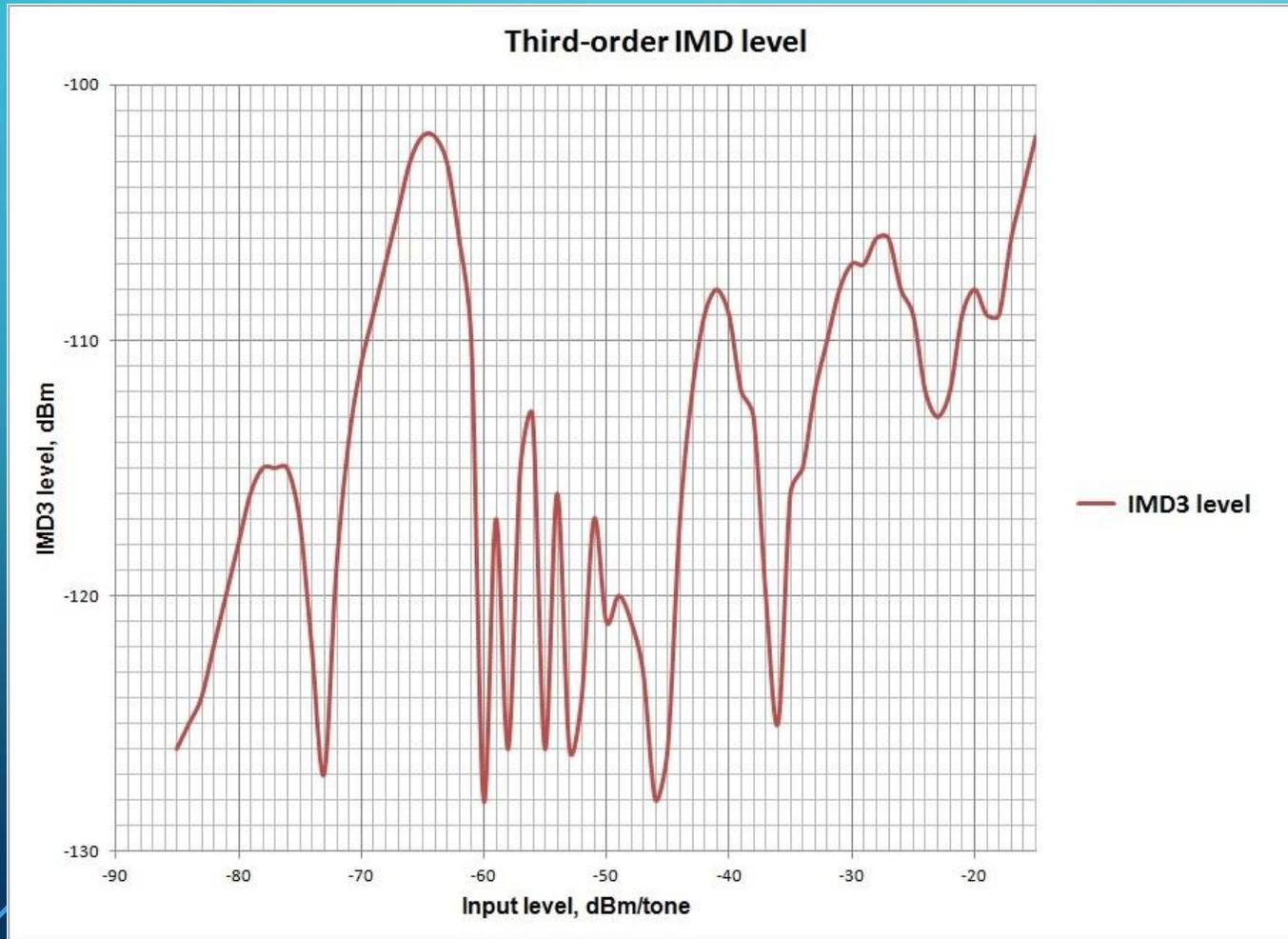
This direct-sampling SDR does post-ADC processing with discrete IC's (DDC, NCO) rather than an FPGA. The gross irregularity of the IFSS curve may be due to processing anomalies in this signal chain at specific input levels.
