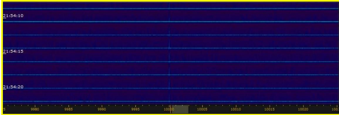
**9. Noise blanker (NB) impulse response:** At the *minimum* NB setting, the AGC pulse response is *completely suppressed*. With NB on, the S-meter reading drops back to the noise floor. Increasing NB level makes no difference to this behavior. (See **Figure 4**.)
