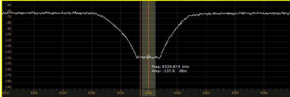
**14. AGC action due to signals outside the channel passband:** The purpose of this test is to determine the input power level at which an unwanted signal falling within the roofing-filter window, but outside the DSP IF passband, starts stimulating the AGC.
