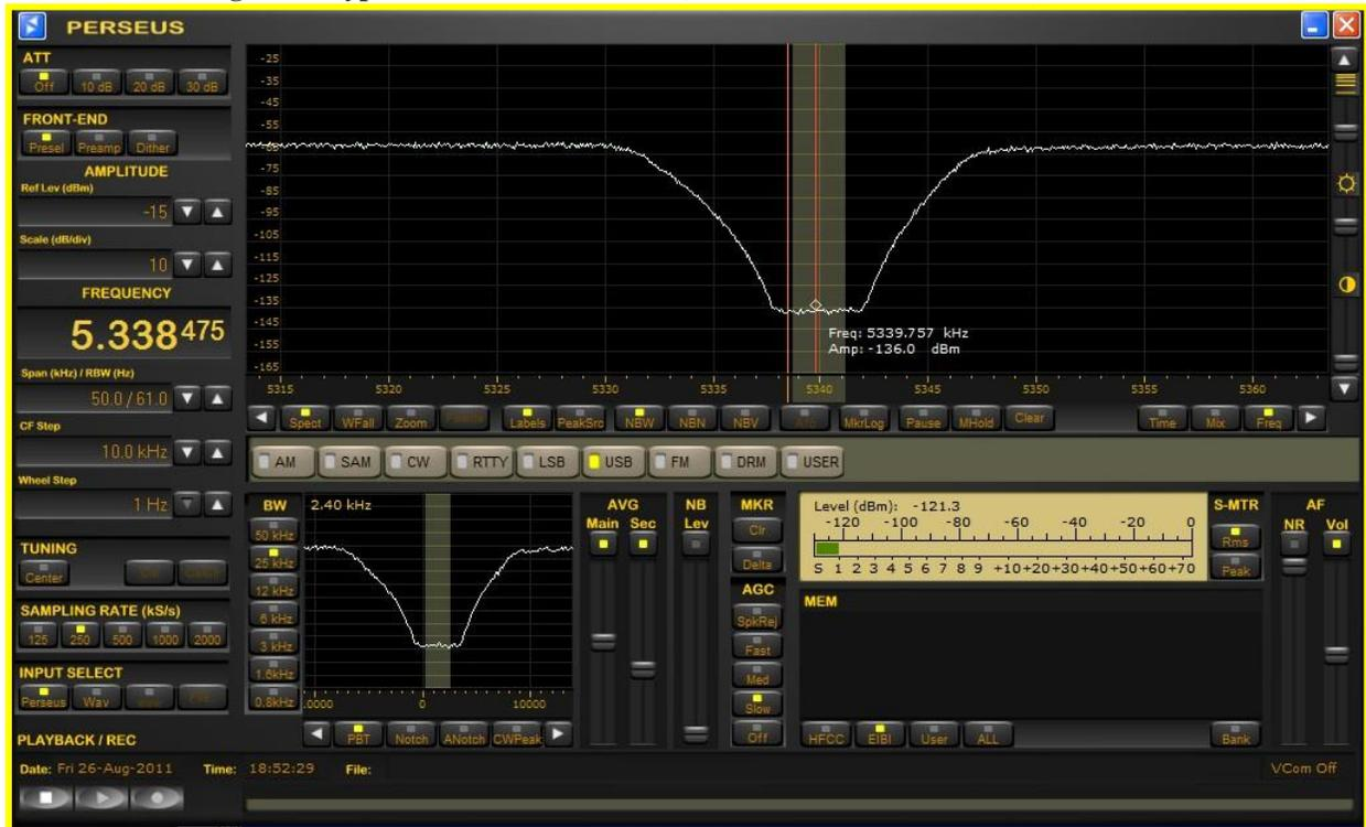
The signal strength meter displays S-units and either dBm or dB $\mu$ V (selectable). The meter is accurate to within  $< 1$  dB; thus, the Perseus is useful as a selective RF power meter covering 10 kHz to 30 MHz.
