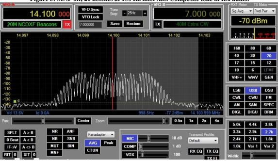
Figure 5: MNF off, 21 notches at 100 Hz intervals. Composite tone in RX audio.
