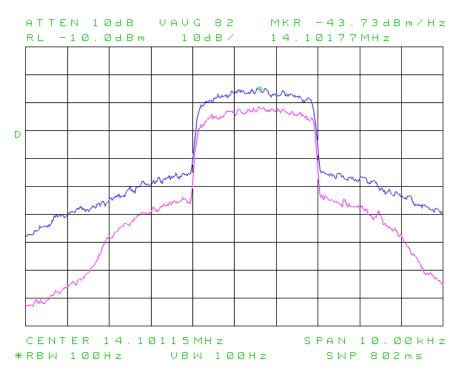
21: AM sidebands and THD with single-tone modulation. As in Test 20 above, the spectrum analyzer is connected to the DUT RF output via a 20 dB 25W attenuator. On the GUI, RF Power is adjusted for 50W resting carrier. A 1 kHz test tone is applied from the internal tone generator. The spectrum analyzer records the carrier and sideband parameters.
