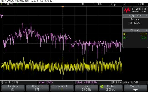
Figure 3: Spectrum and waveform of RX audio with ANF (Pre-AGC). DS0-X 2012A, MY5546213D: Tue Jul 11 12:13:30 2017
