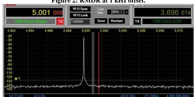
Figure 2: RMDR at 1 kHz offset.
