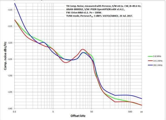
Figure 23: TX composite noise at 3.6, 14.1 & 28.1 MHz, 100W, measured on Perseus RX.
