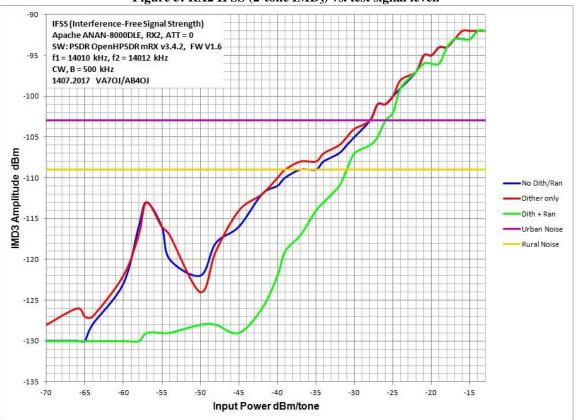
Figure 5: RX2 IFSS (2-tone IMD<sub>3</sub>) vs. test signal level.
