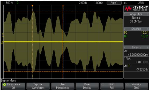
Figure 33: Transmitted RF envelope, USB, 200WPEP, CFC on, VA7OJ Test profile. DS0-X 2012A, MY55462130: Mon Jul 24 15:09:46 2017
