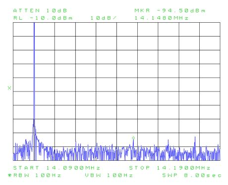
*23: Transmitted composite noise.* A Perseus SDR receiver is connected to the DUT RF output via a 60 dB power attenuator. Figure 23 is the resulting plot.
