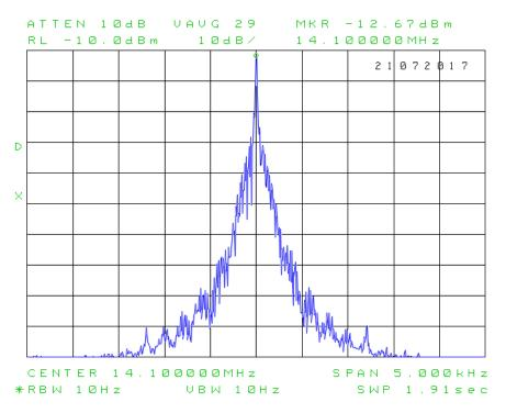
Figure 24: Keying sidebands at 60 wpm, Weight = 50%, 14.1 MHz, 100W. ANAN8000DLE CW spectrum 60wpm dits 2ms delays
