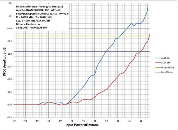
Figure 38: RX1 IFSS (2-tone IMD<sub>3</sub>) vs. test signal level, with ALEX on and off.
