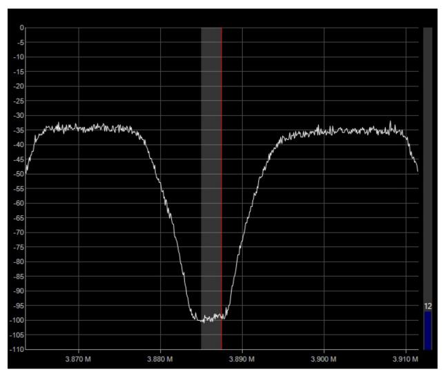
**2.** Sensitivity (MDS): Test setup: HP/Agilent 8935 E6380A, connected to AIRSPY HF+ via a 30 dB fixed attenuator.
