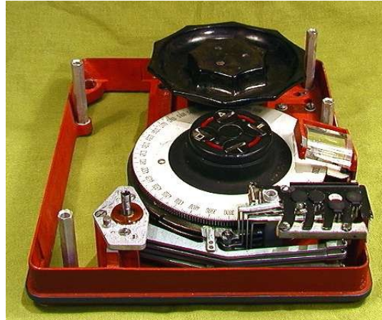
EK front panel frame & tuning dial mechanism with 4 preset cams. Image courtesy LA6NCA
