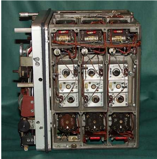
EK Receiver , top view, showing tube sockets, IF transformers and chassis compartments. Image courtesy Bo Samuelsson
