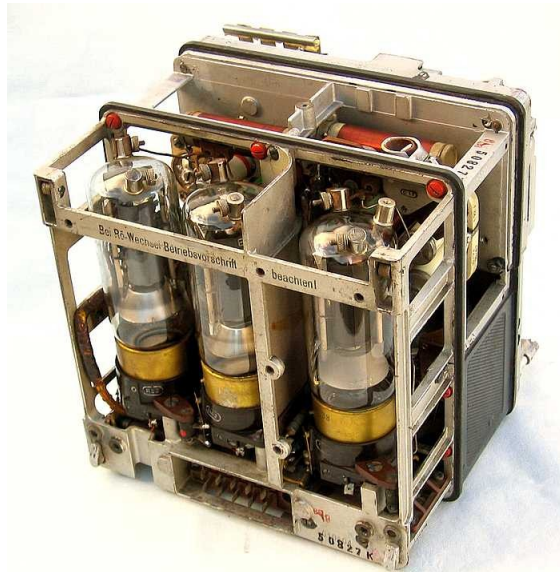
SK Transmitter with RL12P35 tubes (1 in MO, 2 in parallel for PA) Image courtesy LA6NCA
