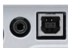
CI-V remote control jack (left) and USB connector on the rear panel ▲
