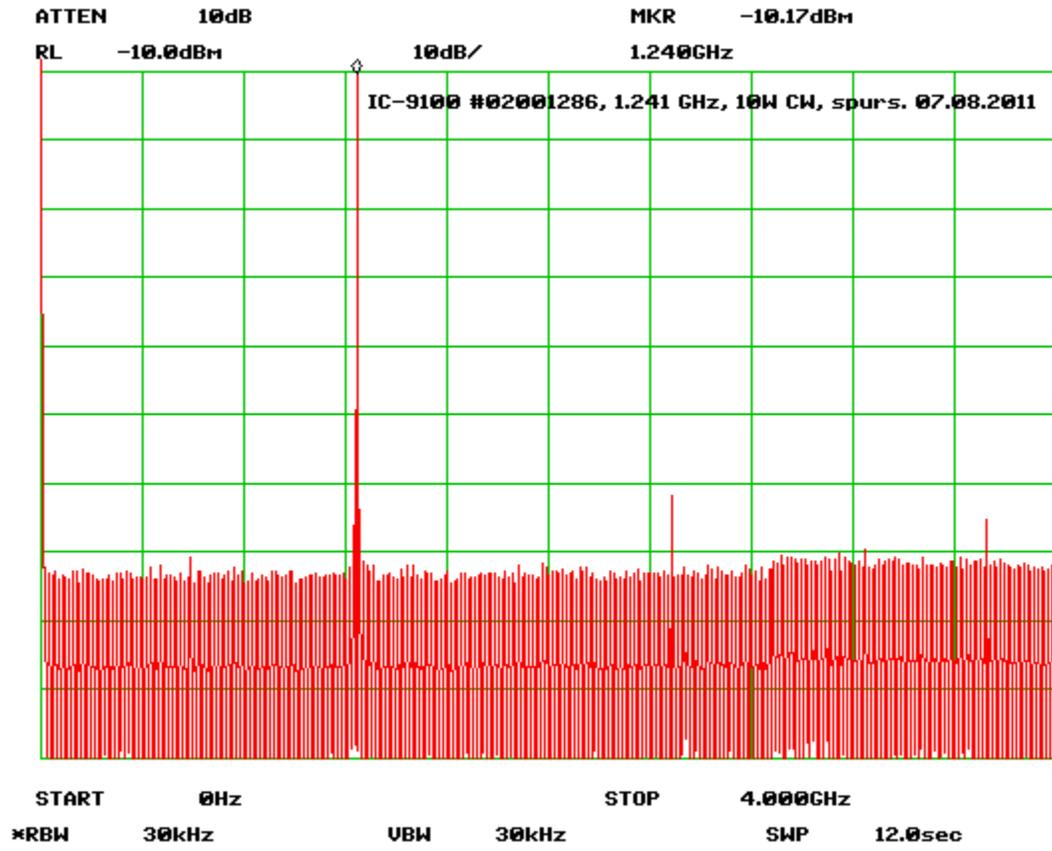
**29: Transmitted composite noise.** The spectrum analyzer is connected to the IC-9100 RF output via a 60 dB high-power attenuator. The spectrum analyzer's phase-noise utility is started. **Figs. 24a** through **24f** are the resulting composite-noise plots.
