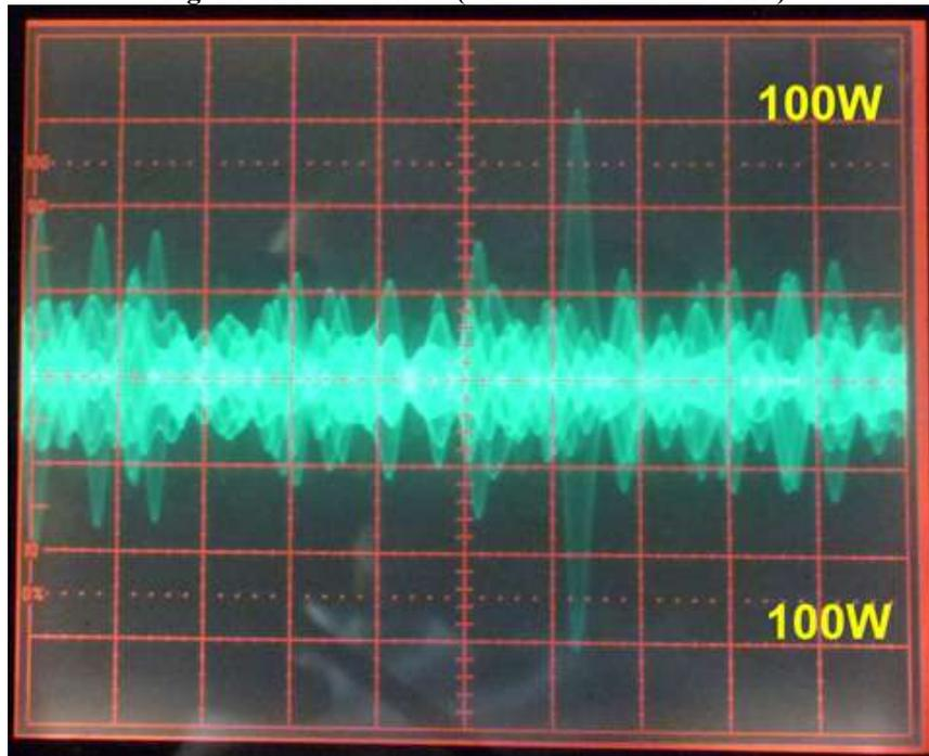
**26: Transmitter 2-tone IMD test.** In this test, a 2-tone test signal is applied to the USB port from a tone-generator program running on a laptop computer. A spectrum analyzer is connected to the IC-9100 RF output via a 50 dB high-power attenuator. RF Power is adjusted for rated CW output on each band in turn.
