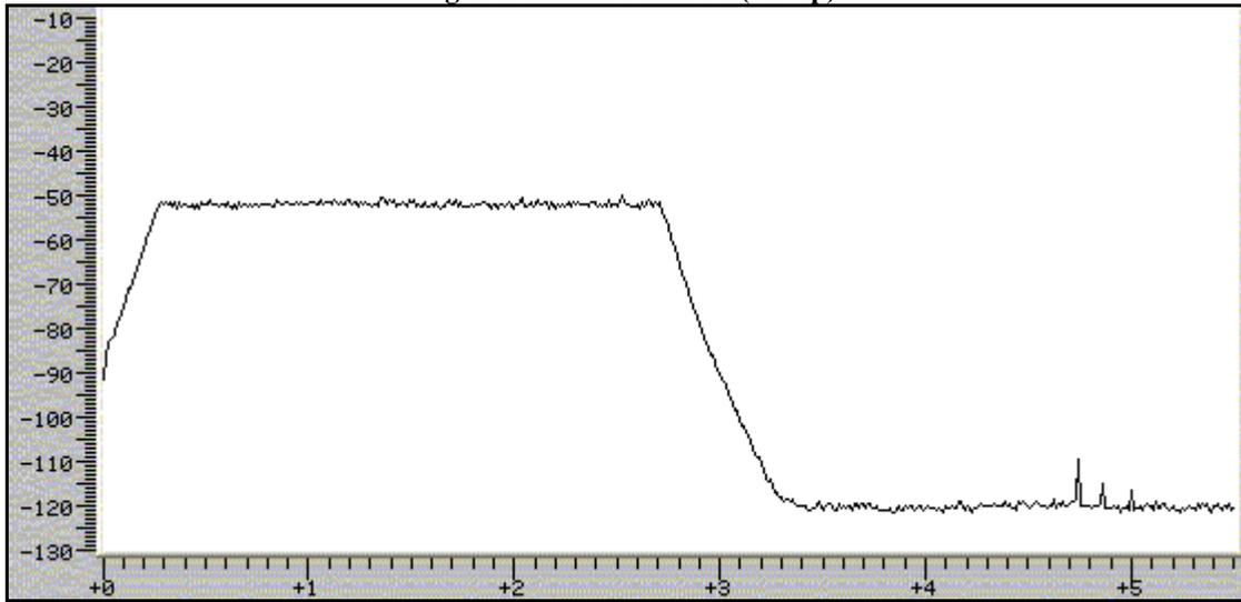
**Fig. 2: 2.4 kHz SSB filter (Soft)**
