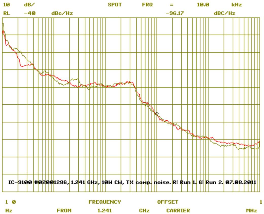
**30: Spectral display of CW keying sidebands.** The spectrum analyzer is connected to the IC-9100 RF output via a 60 dB high-power attenuator. The -10 dBm reference level equates to 100W. A series of dits is transmitted at the highest keying speed.
