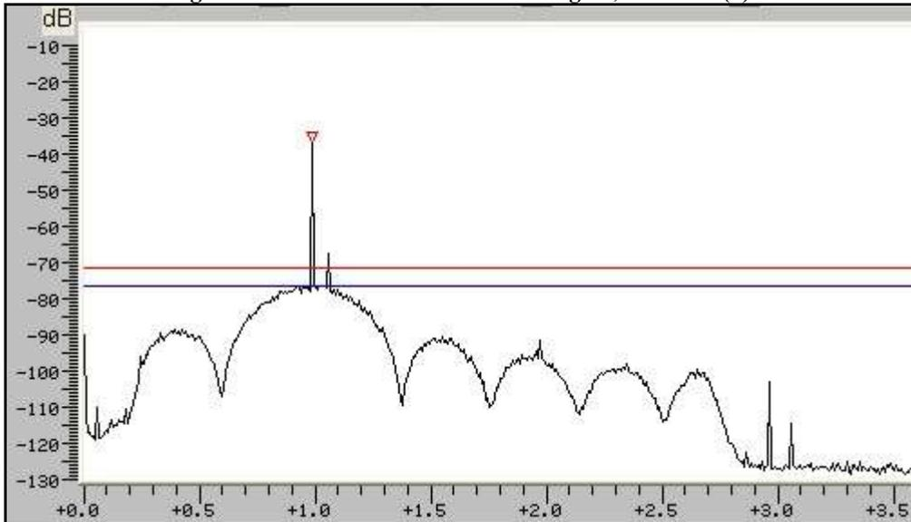
**6: Manual Notch Filter (MNF) stopband attenuation and bandwidth.** In this test, an RF signal is applied at a level  $\approx 70$  dB above MDS. The test signal is offset 1 kHz from the receive frequency to produce a test tone. The MNF is carefully tuned to null out the tone completely at the receiver audio output. The test signal level is adjusted to raise the baseband level 3 dB above noise floor. The stopband attenuation is equal to the difference between test signal power and MDS.
