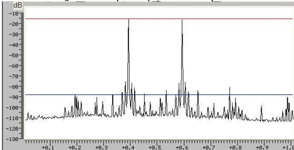
On the X-axis, +0.0 kHz  $\hat{=}$  9999.6 kHz (virtual carrier).  $f_1$  is at +0.4 kHz,  $f_2$  at +0.6 kHz. The 3<sup>rd</sup>-order IMD products are at +0.2 and +0.8 kHz respectively.
