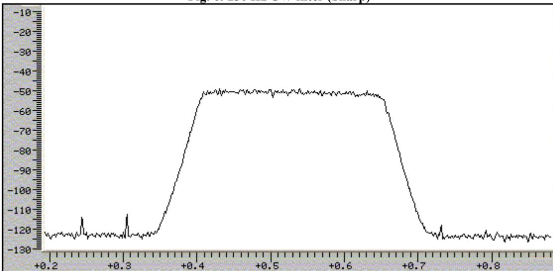
**5: NR noise reduction, measured as SINAD.** This test is intended to measure noise reduction on SSB signals close to the noise level.
