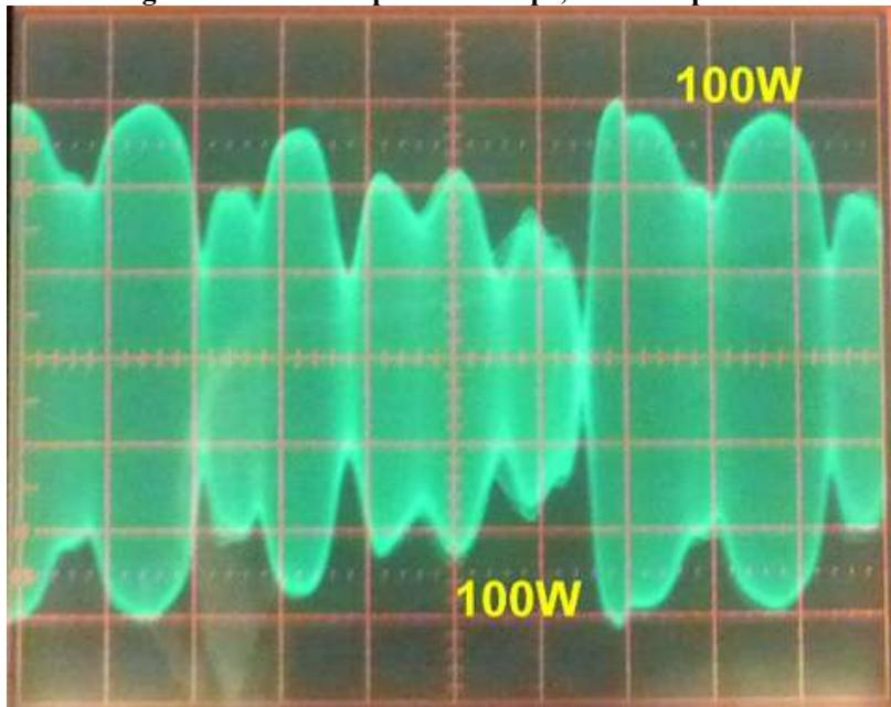
**25: SSB ALC overshoot:** Reports of ALC overshoot in the IC-9100 Yahoo! Group led to an investigation of this issue. A test was performed in which white noise was applied via the USB port, and the RF envelope observed on an oscilloscope terminated in  $50\Omega$  and connected to the IC-9100 RF output via a 50 dB high-power attenuator.
