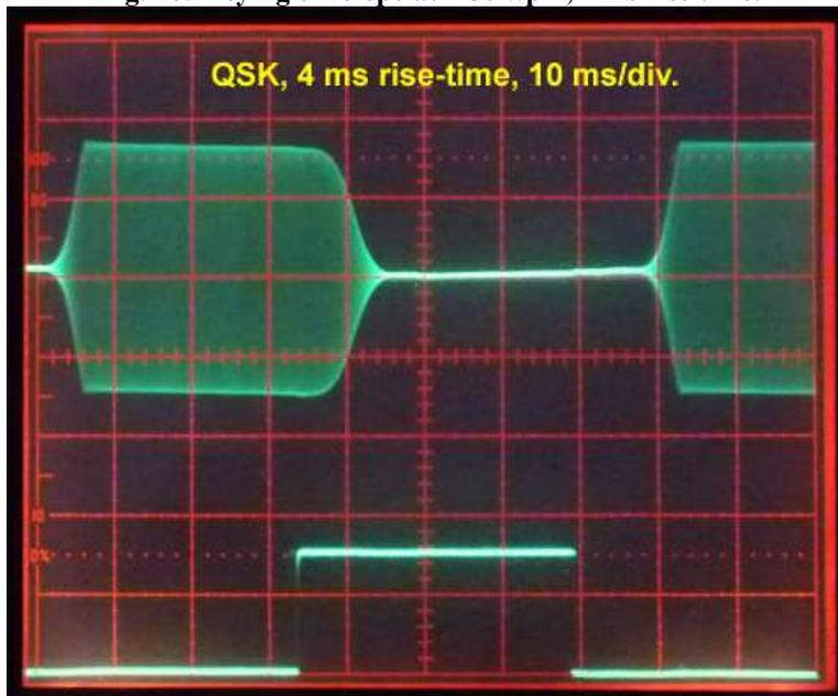
**31b. CW QSK recovery test:** This test was devised to address Yahoo! Group reports that **CW QSK** (full break-in) does not work well when using the internal keyer at speeds > 12 wpm. If a string of dits is transmitted at speeds > 12 wpm, the receiver does not recover between dits.
