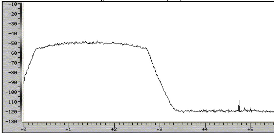
**Figure 3: 500 Hz CW filter (Sharp, BPF)**
