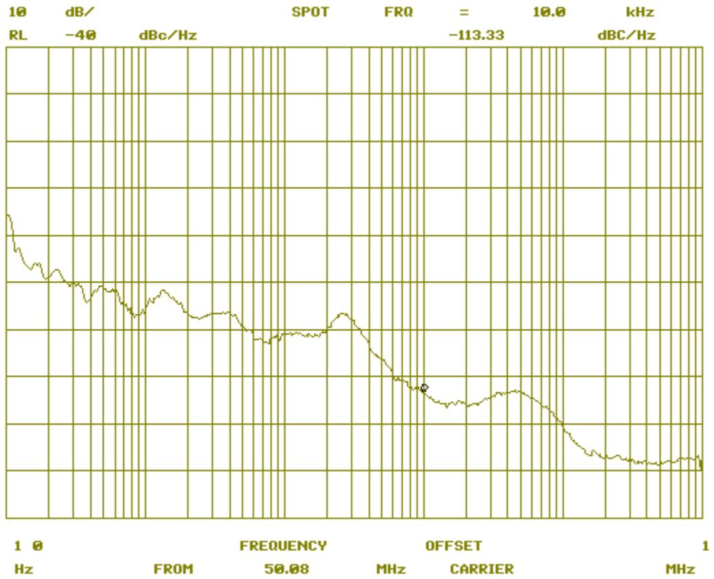
Fig. 24d: Composite noise at 144.1 MHz, 100W.
