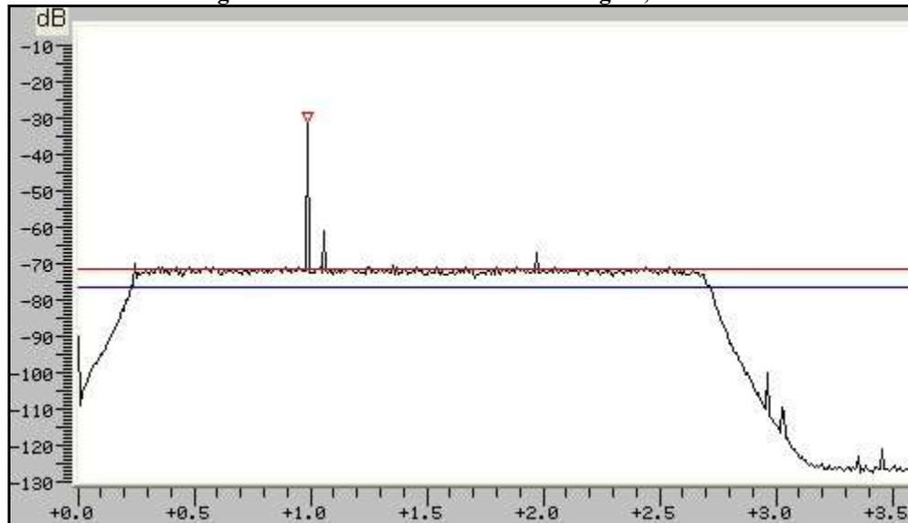
Figure 8: SSB 2.4 kHz. -120 dBm RF signal, max. NR (9).
