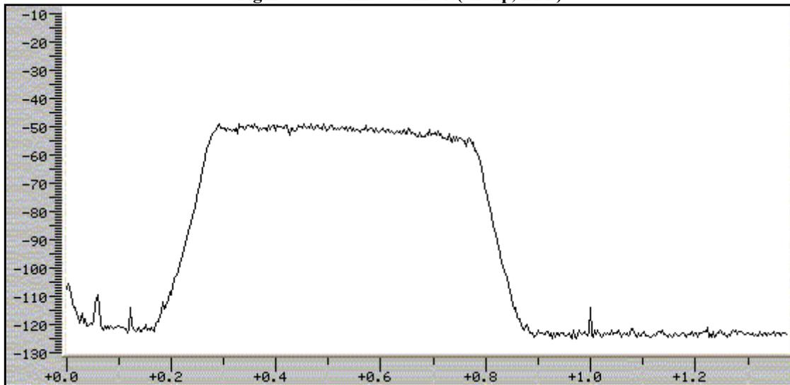
**Fig. 4: 500 Hz CW filter (Sharp, non-BPF)**
