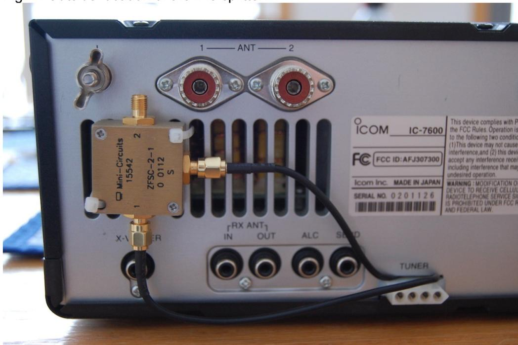
In order to connect the RTL-SDR dongle to the line splitter, I opened the dongle up and removed the original PAL antenna connector. Instead, I soldered in one of the RG174 SMA cables and hooked it up to Port 2 of the splitter (Fig 5).
