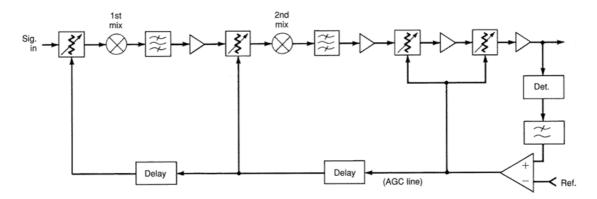
**Figure 4.13** A double-conversion receiver has distributed AGC attenuators to prevent stage overload while also causing the output signal-to-noise ratio to rise with signal increases.
