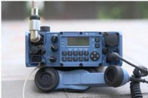
**Figure 1** R&S®MR3000U manpack radio, covering 25 to 512 MHz.
