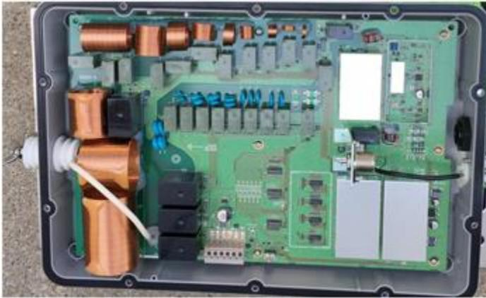
**Figure 16** ICOM antenna tuner with 90 degree offset coils.
