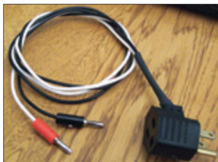
Figure 4 — The completed current measuring adapter. [David Stein, KC9NVP, photo]
