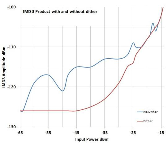
Dither breaks up IMD products into noise which degrades RX noise floor by • 3 dB. Courtesy HB9CBU
