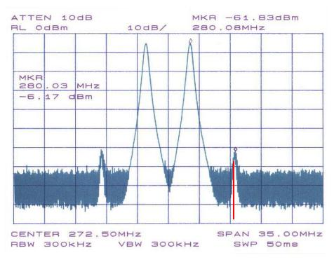
IMD Example:  $f_1 = 270 \text{ MHz}$ ,  $f_2 = 275 \text{ MHz}$ .
