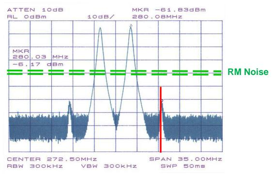
IMD Example:  $f_1 = 270 \text{ MHz}$ ,  $f_2 = 275 \text{ MHz}$ .
