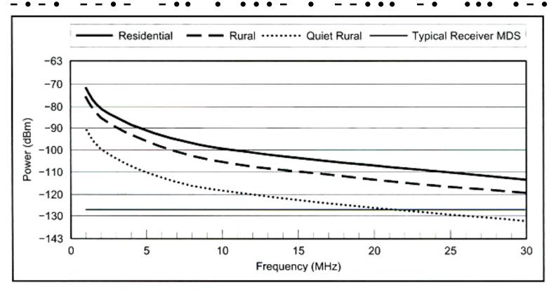
Typical noise levels versus frequency for various environments. (Man-made noise in a 500-Hz bandwidth, from Rec. ITU-R P.372.7, Radio Noise)
