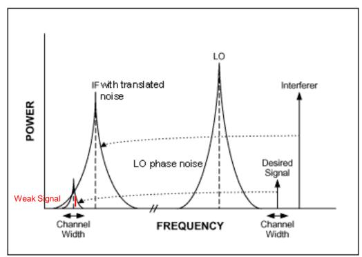
Strong interferer mixes with LO phase noise to "throw" noise into IF channel. If the interferer consists of wideband noise, the IF channel will be filled up with noise.
