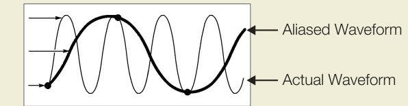
■ To avoid aliasing, the oscilloscope must sample the signal more than twice as fast as the highest frequency component of the signal (Nyquist Theorem). Tektronix oscilloscopes sample at least five times as fast as their highest bandwidth, substantially minimizing the chance of aliasing.
