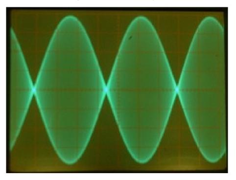
Figure 7: 2-tone RF envelope at 81W PEP (measured). Note ALC compression on peaks.
