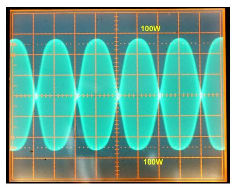
**Test B3c: ALC compression tests using white noise:** The test instrument (oscilloscope terminated in 50 $\Omega$ , then spectrum analyser) is cnnected to the DUT RF output via the power attenuator. The tone/noise generator program in the connected laptop feeds white noise to the DUT USB port.
