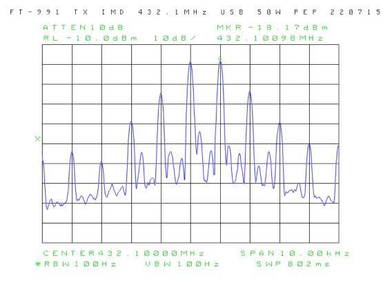
**Test B5: Transmitted composite noise.** As before, the The spectrum analyser is connected to the DUT RF output via the power attenuator. The spectrum analyser's phase-noise utility is started. Figures 12a through 12c are the resulting composite-noise plots. (*Note:* The limitation of this measurement method is that the lowest values of measured noise power are close to the spectrum analyser's own noise floor.)
