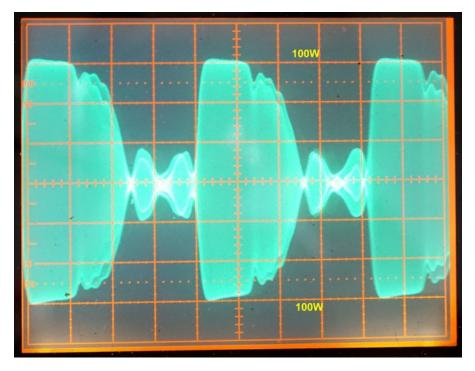
Figure 5: SSB RF envelope at 100W PEP nominal (81W PEP measured), 0% ALC. No ALC compression.
