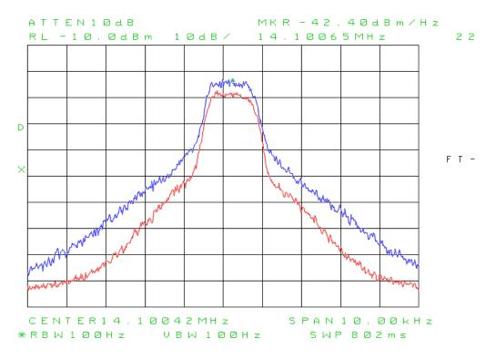
**Test B4: TX IMD test using 2-tone test signal:** The spectrum analyser is connected to the DUT RF output via the power attenuator. The tone/noise generator program in the connected laptop feeds the 2-tone test signal to the DUT USB port. Figures 11a through 11e are the test plots.
