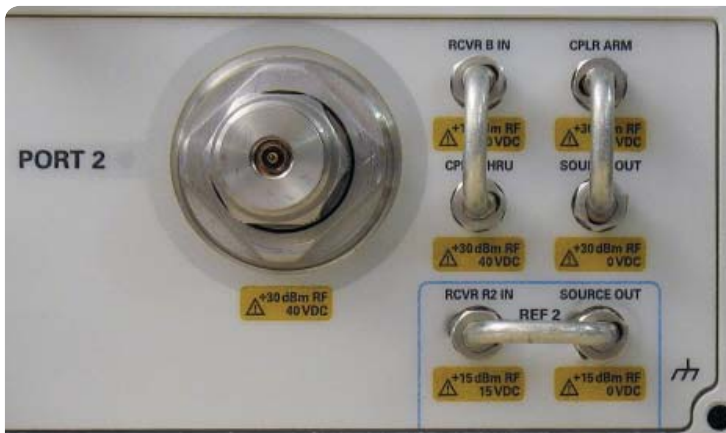
Figure 30. Jumper cable arrangement for reversing the test port coupler (main and coupled arms swapped)
