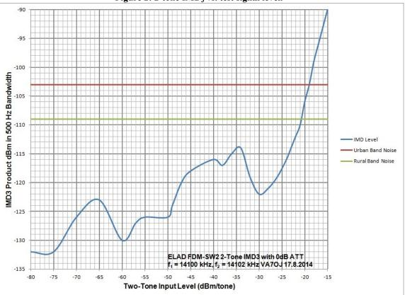
Figure 2: 2-tone IMD<sub>3</sub> vs. test signal level.
