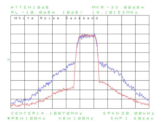
Figure 27: Wideband TX noise floor with PureSignal off/on, 100W.
