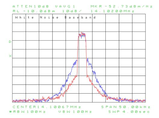
Figure 5: TX composite noise at 14.1 MHz, 30W.
