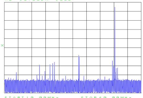
START 1 0 . 0 0 MHz STOP 6 0 . 0 0 MHz #RBW 3 . 0 kHz VBW 3 . 0 kHz SWP 1 4 . 0 sec
