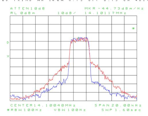
Figure 4a: White Noise IMD at 14.1 MHz, 100W PEP, PureSignal (PS) off & on (Test 9a, 50 kHz). A N A N 2  $\ 0\ 0\ D$  1  $\ 0\ 0\ W$  P E P B : P S o f f R : P S o n  $\ 0\ 7\ 1\ 0\ 1\ 4$
