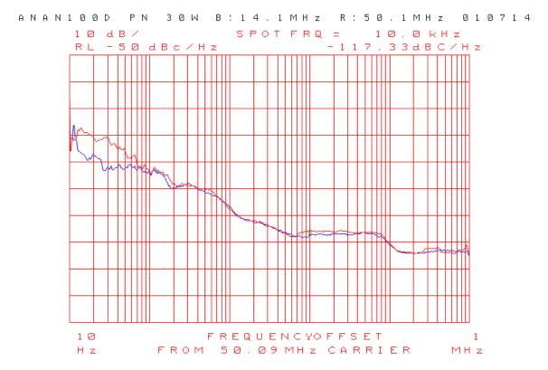
21: Spectral display of CW keying sidebands. The spectrum analyzer is connected to the ANAN-100D RF output via a 60 dB high-power attenuator. The -10 dBm reference level equates to 100W. A series of dits is transmitted at 60 wpm.
