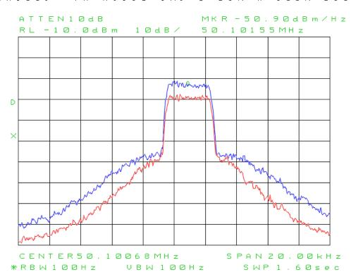
18: AM sidebands and THD with single-tone modulation. As in Test 17 above, the spectrum analyzer is connected to the ANAN-100D RF output via a 50 dB high-power attenuator. On the ANAN-100D, RF Power is adjusted for 25W resting carrier. A 1 kHz test tone is applied from the internal tone generator. The spectrum analyzer records the carrier and sideband parameters.
