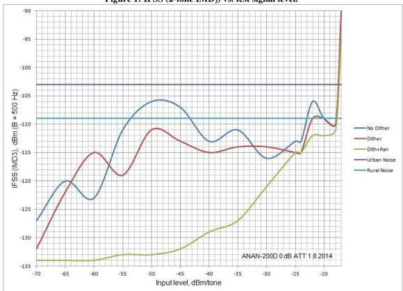
Figure 1: IFSS (2-tone IMD<sub>3</sub>) vs. test signal level.
