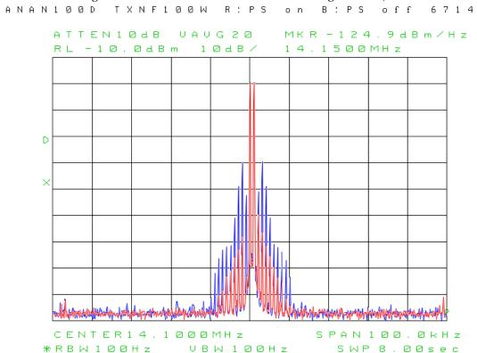
Figure 28: AM Sidebands for 90% Modulation, PureSignal on. THD  $\approx$  0.2%.
