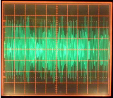
**16. ALC Compression Check.** In this test, a 2-tone test signal is applied to the USB port from the internal 2-tone generator. An oscilloscope is connected to the ANAN-100D RF output via a 50 dB high-power attenuator. RF Power is initially adjusted for 100W CW output.
