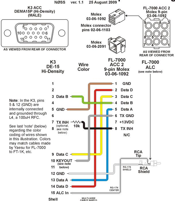
**KEYOUT** (K3 ACC pin 10) should sink no more than 10mA of current to ground. If you must key >10mA of current, use the separate **KEY OUT** jack on the rear of the K3.
