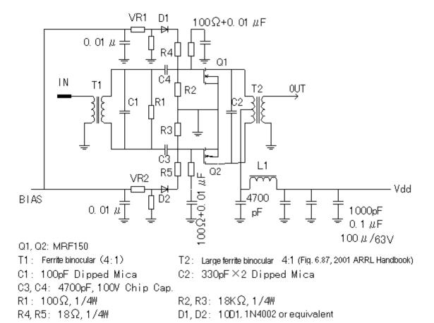
This module is rated at 250W output. Two or four identical modules may be combined via an input splitter and output combiner for 500W or 1kW output.
