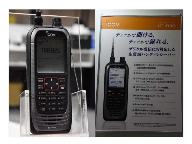
The IC-R30 is the successor of the IC-R20 wide band, all mode receiver. The IC-R30 has additional digital modes built-in, and simultaneous two band reception. The receiver covers 100kHz to 3.3GHz for super wide band reception.
