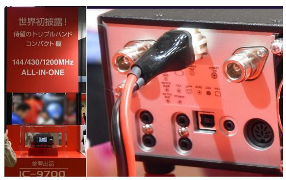
You can see connectors on the rear panel through the display back mirror. There are several connectors for LAN, DATA, USB and REMOTE.
