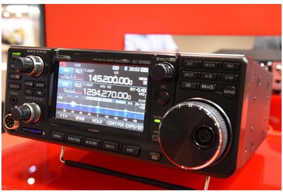
The concept model IC-9700 is the same size as the popular IC-7300, but covers the 144, 430, and 1200MHz bands. The transceiver operates on all the standard modes, as well as the DD mode on D-STAR. It has simultaneous two band reception, with some limitations, a touch-panel screen, satellite mode, and so on. It should be a very popular model if it is released.
