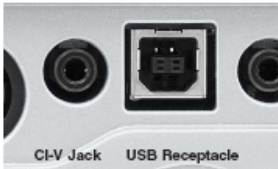
The IC-9100 has a standard type B USB connector for rig control as well as modulation input, audio output, RTTY demodulator output and CI-V command can be controlled via the USB cable.
