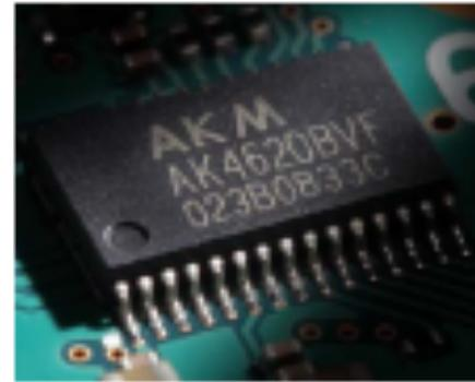
Employing the ADSP-21369 (DSP) and AK4620 (AD/DA) to provide a powerhouse of DSP performance in a HF/6m/2m/70cm Rig.
