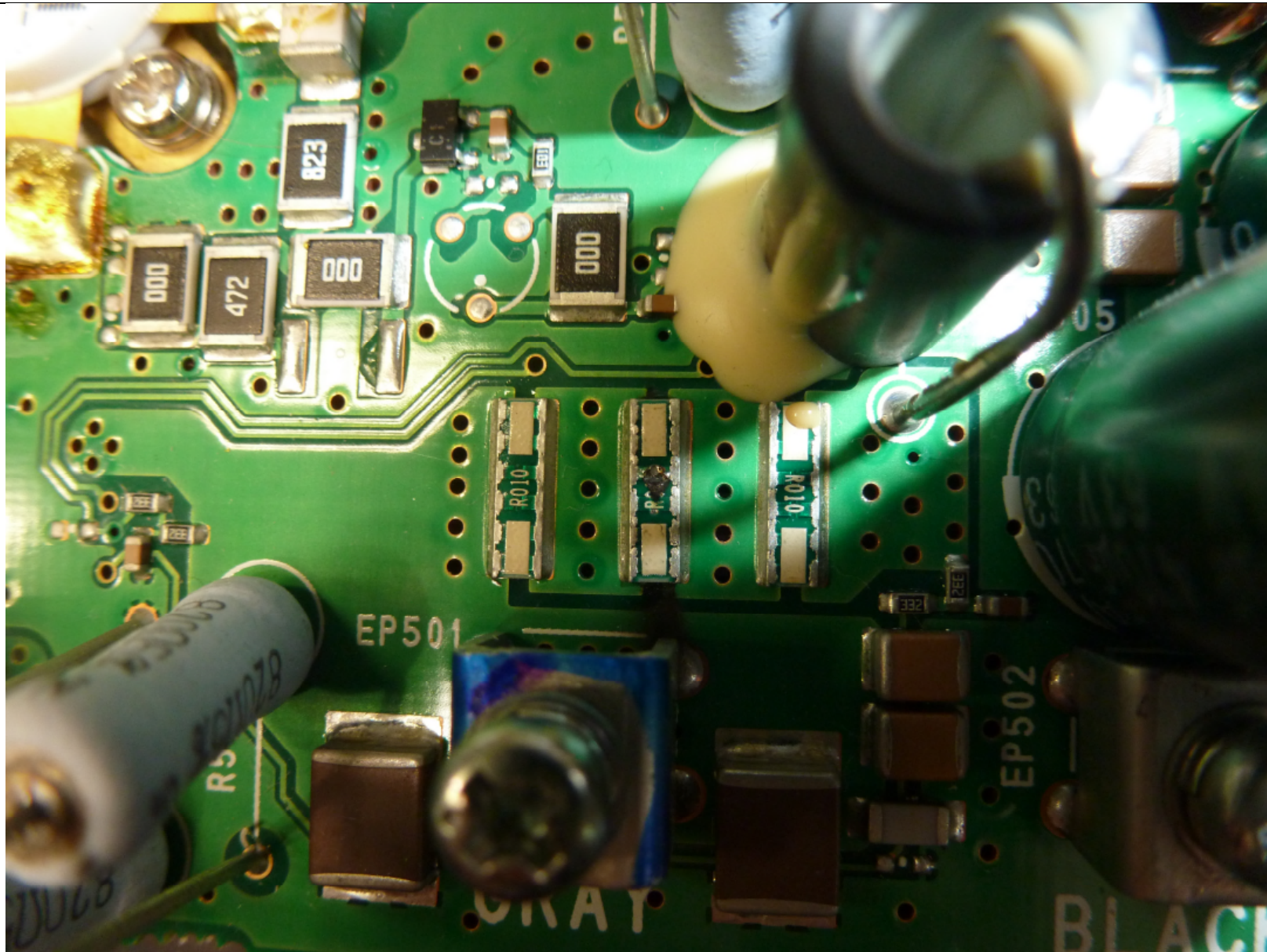
Two of three shunt are blowing (three times 10 mΩ in series connection = 30 mΩ)
