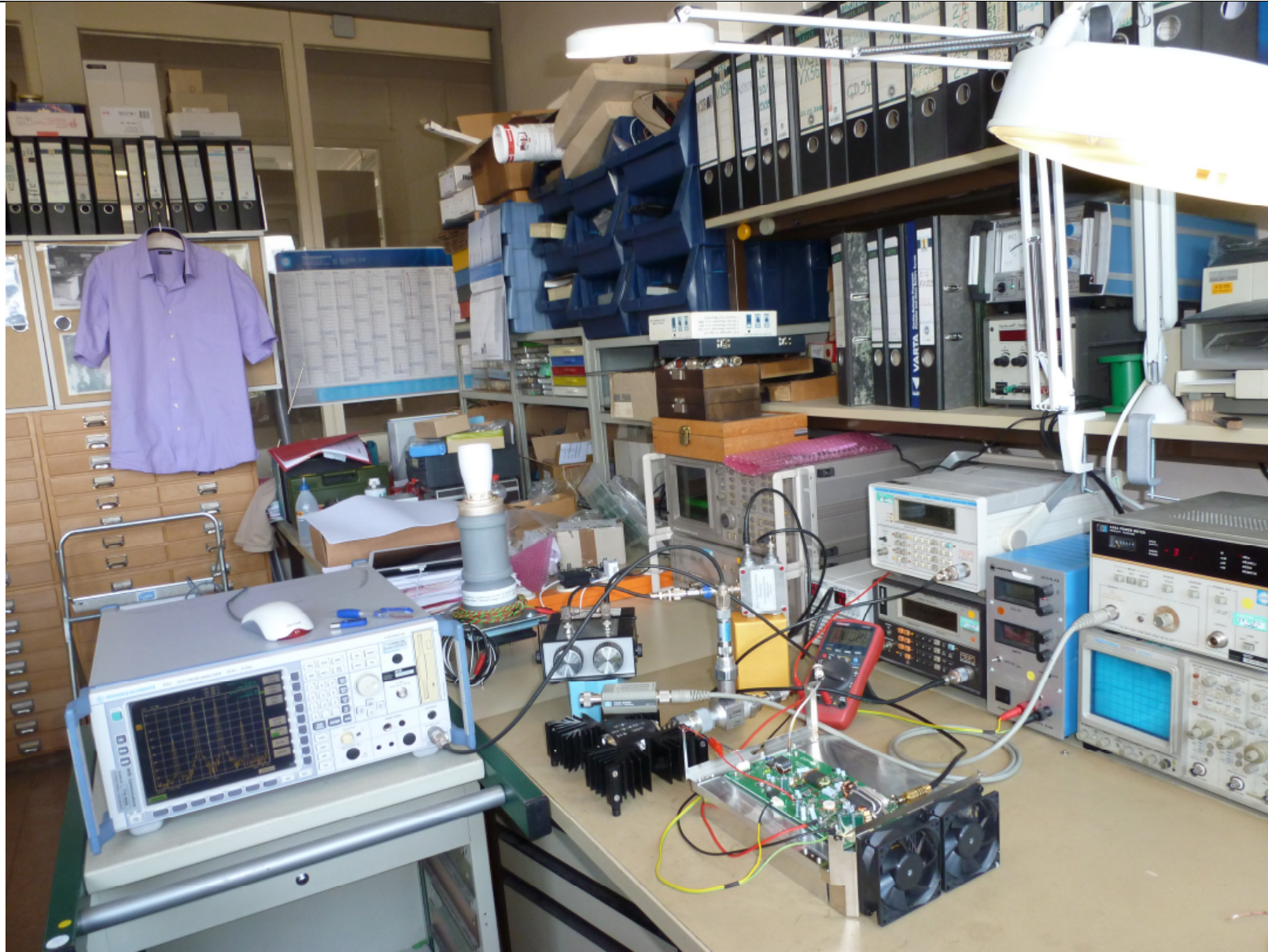
Preparation for measurement the third order IMD
