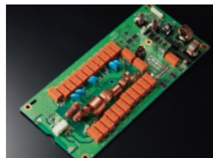
Antenna tuner unit
