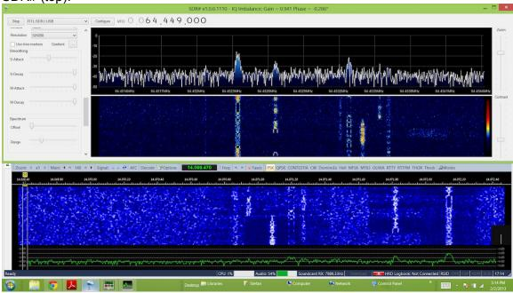
If you look carefully at the picture in Fig 6, you will see that the image in SDR# is initially mirrored. By checking the Swap I&Q button (in SDR#), this can be undone and any tuning on the radio will move the signal on both (HRD and SDR#) in the same direction.
