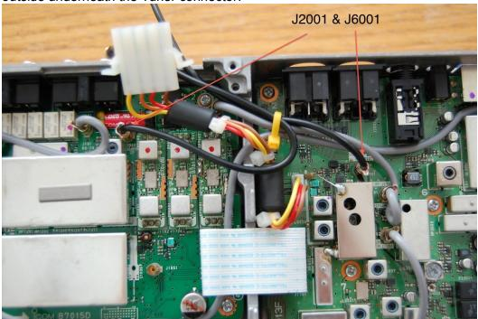
I mounted the line splitter with two cable ties on the outside of the radio (again, no drilling or permanent modifications) and hooked up the two cables. The J2001 cable goes into the S (signal) port of the splitter and the other cable goes to port 1. Port 2 gets connected to the dongle (Fig. 4).
