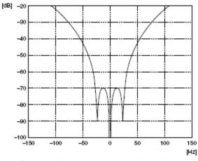
Characteristics of manual notch (enlarged view)
