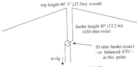
Finally, if you want to use it on other HF bands (3.5, 10,21 MHz), an ATU (just like at the bottom of your '5R V !) will do the business, but preferably at the bottom of the 450 ohm feeder with a balanced output, not after a length of 50 ohm coax, if you've had to use it to reach your rig. Of course for 1.8 MHz (160m), you could short out the feeder twin, and feed it like a Marconi antenna, with a suitable ATU. Not very clever, however.
