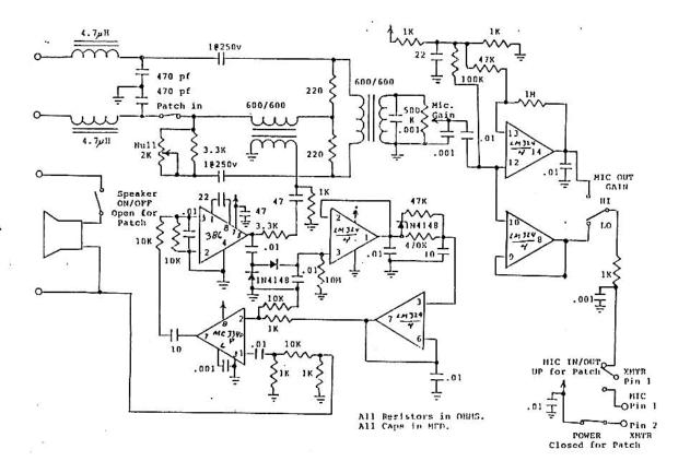
Figure 1. Schematic Diagram of Icom PP-1 Phone Patch.
