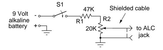
Figure 3: QRP adaptor for IC-765
