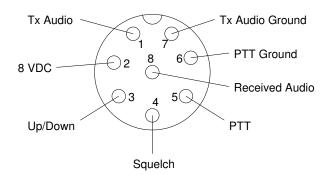
Figure 11: Microphone connectors. (Chassis connector as viewed from outside).
