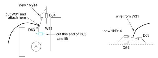
Figure 1: PBT modification top and side views.
