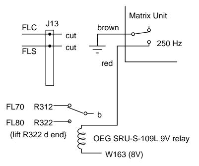
Figure 5: Circuit After Modification
