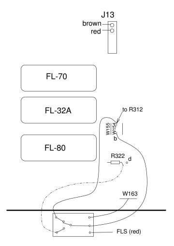
Figure 6: Pictorial of the Filter Modification
