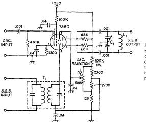
Fig. 4— Balanced mixer circuit with separate excitation. Capacitances are in  $\mu f_{*,i}$  fixed resistors are  $\frac{1}{2}$  watt except as indicated. Tuned-circuit constants depend on frequency; ordinary L/C ratios may be used for  $L_1C_1$  and in the s.s.b. input transformer,  $T_1$ .  $R_1$  is a linear-taper composition potentiometer.
