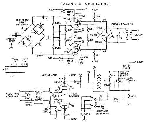
Fig. 5—Phasing-type s.s.b. generator using two 7360s as balanced modulators. Capacitances are in  $\mu\mu$ f.; fixed resistors are  $\frac{1}{2}$  watt except as indicated.
