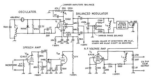
Fig. 2—Filter-type s.s.b. generator using the 7360 as a combined self-excited oscillator and balanced modulator. Fixed resistors are ½ watt except as indicated.
