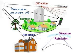
Figure 1.3: Radio wave propagation phenomena
