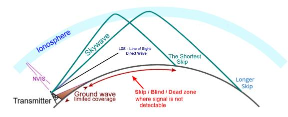
Figure 4.1: **Overview of HF Propagation Modes** In chapters 7-9, we explore the factors and conditions that influence skywave propagation.
