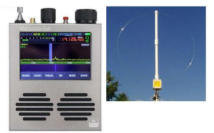
Figure 2.5: **Malahite v1.3 DSP Receiver** connected to <u>K-180WLA</u>—Receive-only **Magnetic Loop antenna** (MLA) **WSPR** <u>∠</u> (Weak Signal Propagation Reporter) is used to test propagation paths on the <u>ham</u> <u>bands</u>. The following are useful links: <u>WSPRnet</u>, <u>WSPR Rocks</u>, <u>WSPR Live</u>.
