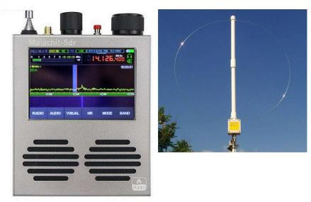
Figure 2.5: **Malahite v1.3 DSP Receiver** connected to K-180WLA **Magnetic Loop antenna** (MLA)
