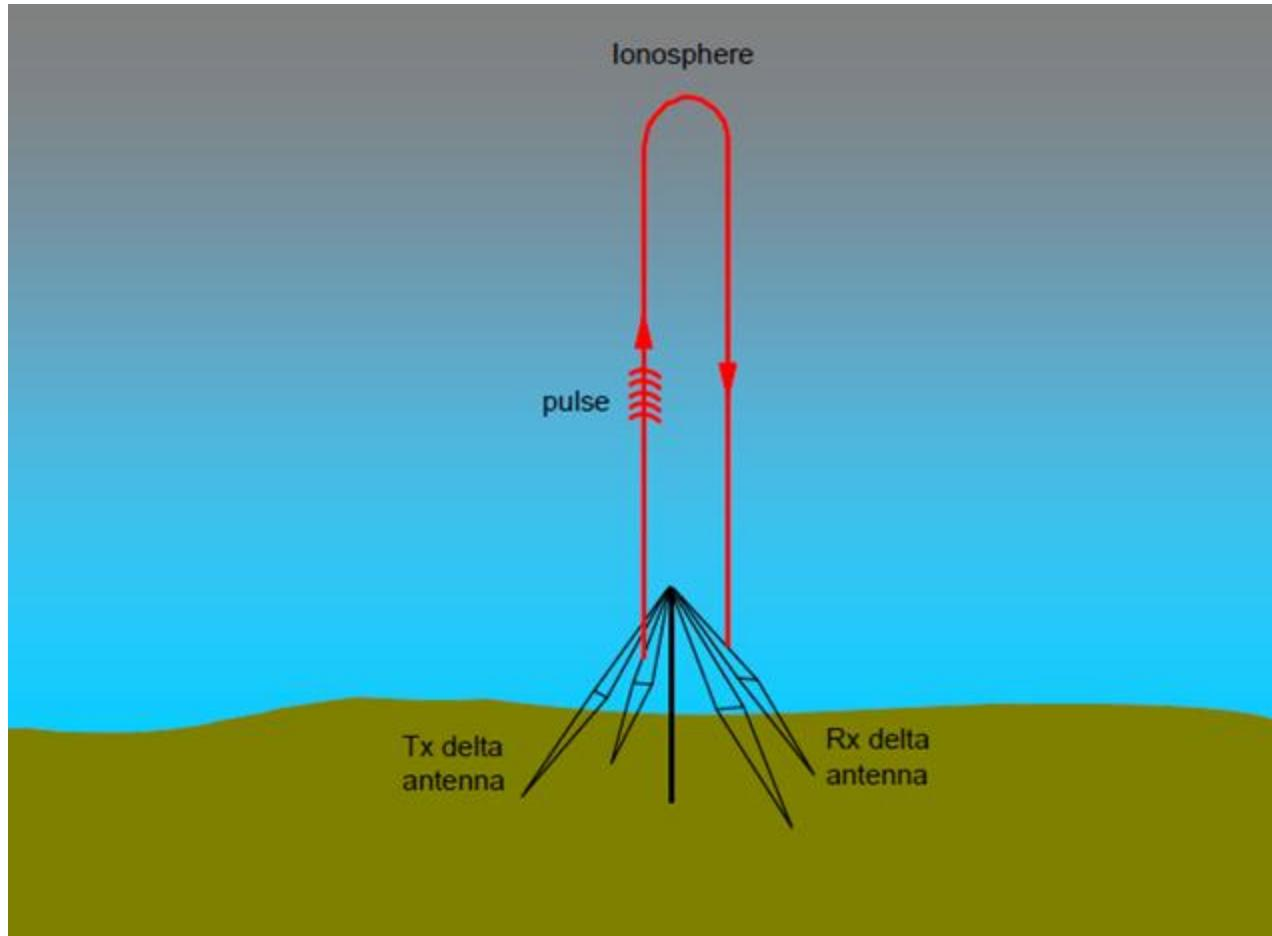
A basic schematic of an ionosonde | The Planetary Society
