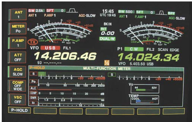
Figure 7—The display providing a view to all metering functions simultaneously.
