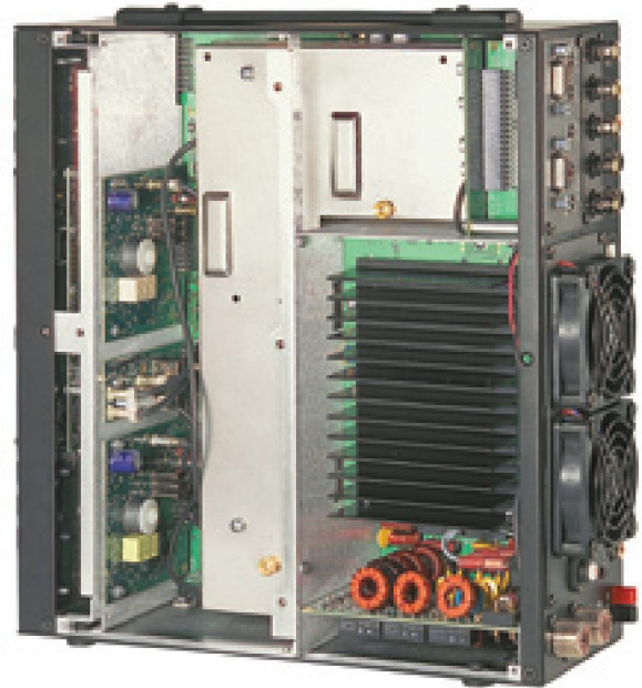
Figure 5 — Interior view of the K3/100. The 100 W output stage is shown in the center rear. The subreceiver occupies the L shaped enclosure filling the front portion of the inside of the radio. Removing the two knurled nuts and three miniature coax connections allows the subreceiver to be easily removed to add main receiver roofing filters, for example.
