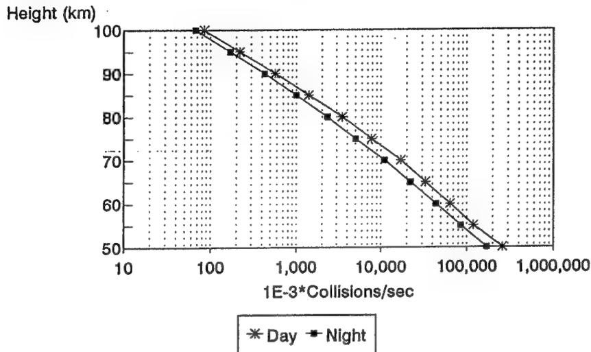
Figure 13 - Electron-neutral collision frequency profile for solar minimum.
