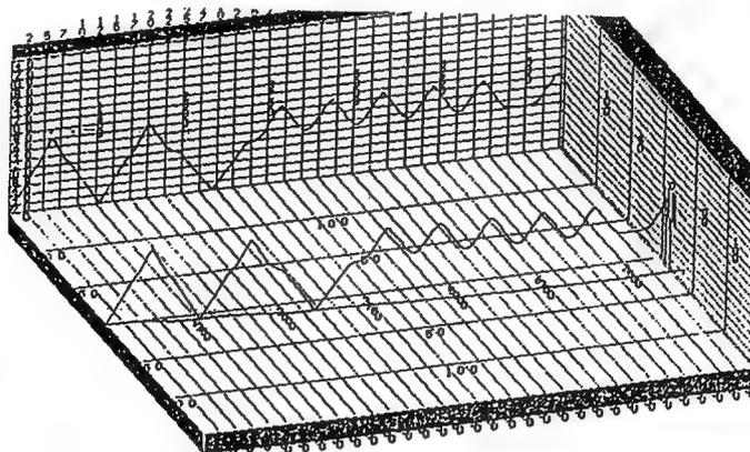
Figure 59 - Tokyo-Seattle ray-trace for "with field" condition.
