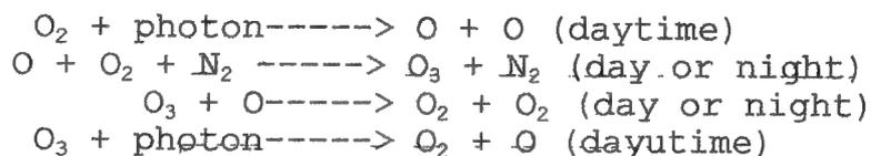
In the absence of sunlight to dissociate ozone and end atomic oxygen creation at night, the ozone in the atmosphere lingers til dawn when the cycle starts all over again. But ozone remaining at dawn is important to low-band operators, as may be seen from another process in the ionosphere, the formation of negative ions at night.
