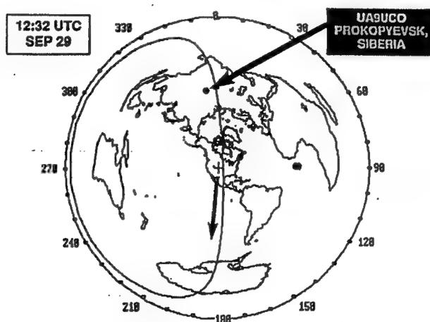
Figure 83 - Azimuthal map with arrow showing the suggested path from WOZV in Colorado to UA9UCO in Siberia.
