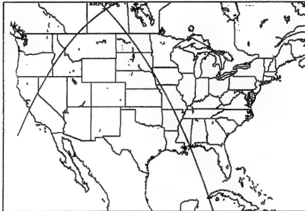
Figure 64 - Dead zone for 1.8 MHz signals from VK0IR.
