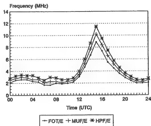
Figure 28 - FOT/E, MUF/E and HPF/E for Boulder-London path.
