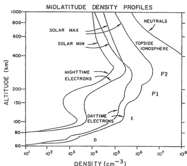
Figure 1 - Ionization profiles for ionospheric layers
