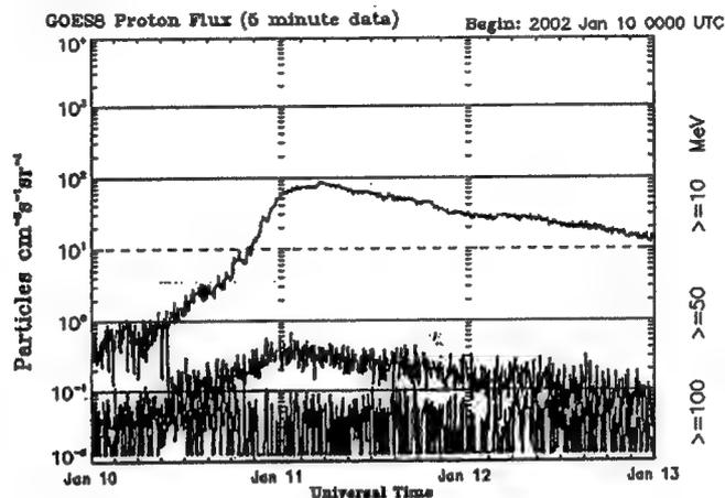
Figure 66 - The particle fluxes in a gradual proton event.
