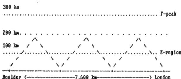
Figure 20 - Reflection path from Boulder to London.
