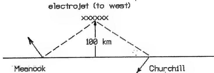
Figure 75 - Magnetic disturbances from a westward electrojet.
