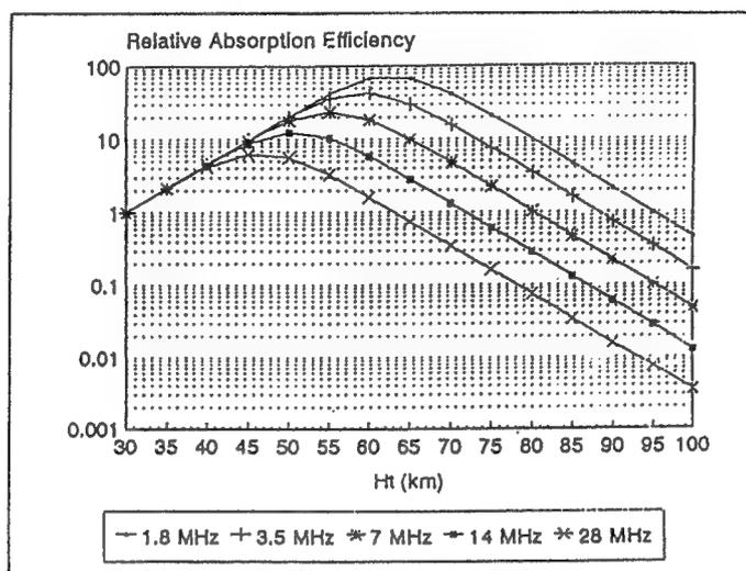
Figure 14 - Relative absorption efficiency per electron
