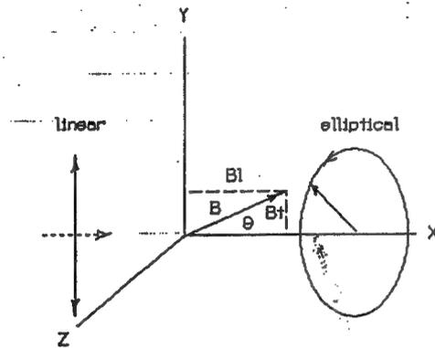
Figure 51 - Near-circular polarization from quasi-longitudinal (QL) propagation ( $B_t \ll B$ ).
