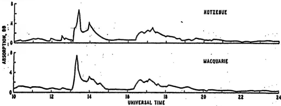
Figure 92 - Absorption records of riometers located at conjugate points in the geomagnetic field.
