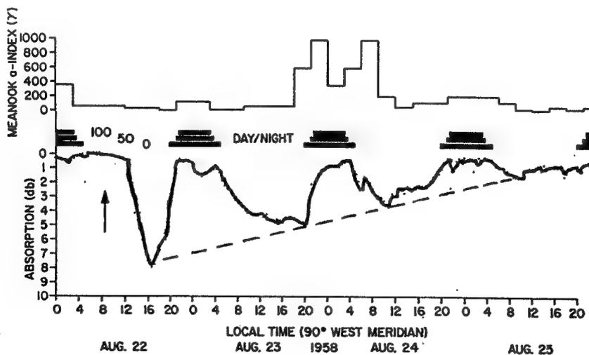
Figure 67 - Ionospheric absorption (down) in a proton event.
