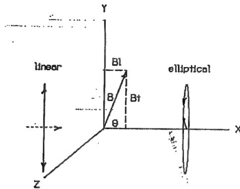
Figure 50 - Elliptical polarization from quasi-transverse (QT) propagation ( $B_l \ll B$ ).
