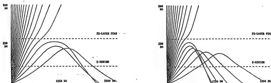
Figures 31 and 32 - Ray-tracings for 14 and 21 MHz signals, with rays going from 5 to 90 degrees in 5 degree steps.
