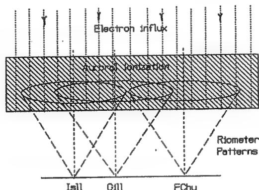
Figure 76 - Auroral ionization relative to riometer antennas.
