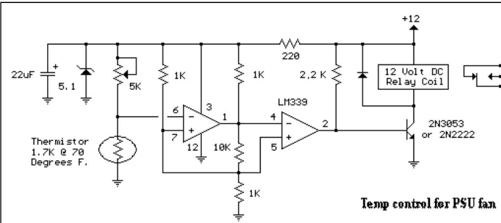
We present yet another quick and effective temperature controlled fan design. The concept is that the first Op-Amp is used as an voltage comparator. Thus the voltage across the thermistor is compared to the preset of the 1k on pin 7. the second Op-Amp acts as an inverting buffer amp that deliver around 20mA to the transistor and activates the relay. The contacts is that used to control any installed fan.— ed.
