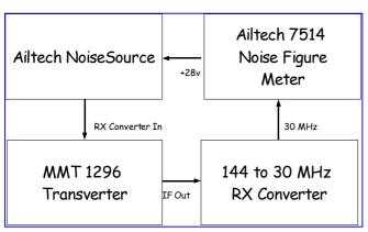
and Filter PCB's. The FET is self biased using bypassed source resistors. These changes resulted in a new converter noise figure of 1.6 dB and just over 2 dB via the PIN diode switch.
