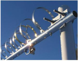
When built up, the 23cm Loop Yagi has the following performance:
