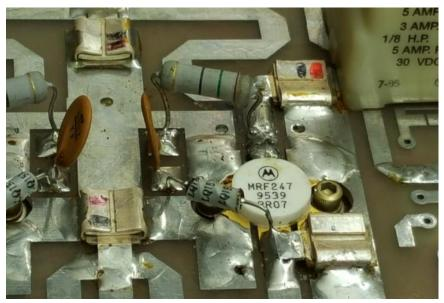
With the south amplifier repaired, SWR checks on the feed lines showed minimal reflected power on both north and south arrays. Thanks to Harry ZL1BK, we had his spectrum analyser on site and the return loss measured at -16dB. This equates to an SWR of just over 1.3:1, an acceptable value. The 2m D-Star antenna gave a return loss of -15dB.
