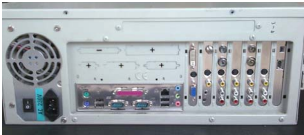
Photo is of back-panel with four AV inputs
