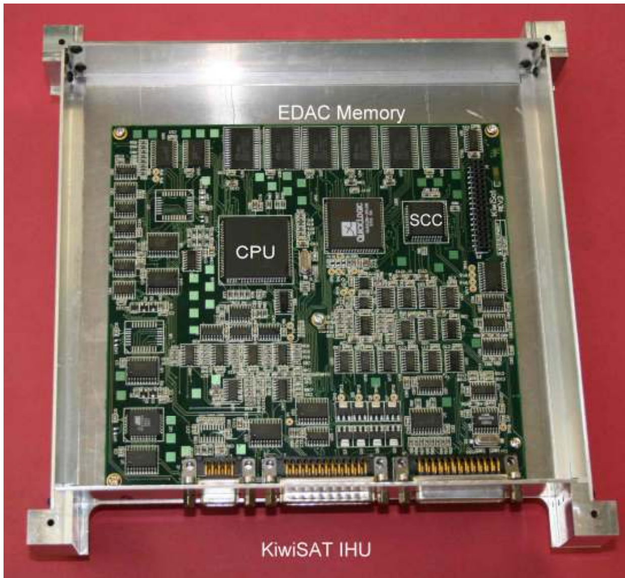
KiwiSAT IHU in temporary tray
