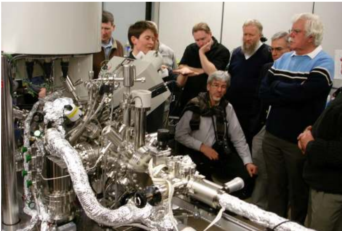
X-ray Spectroscopy. Sample is held in tube at right
