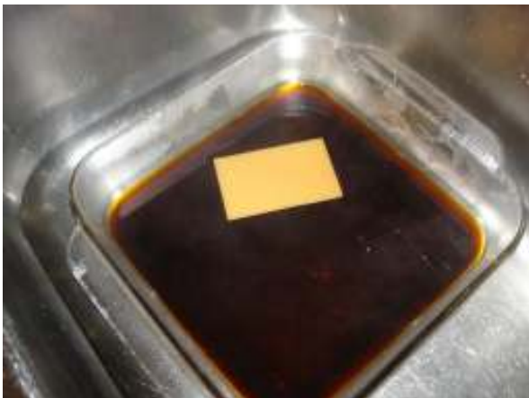
PCB floating on ferric Chloride solution
