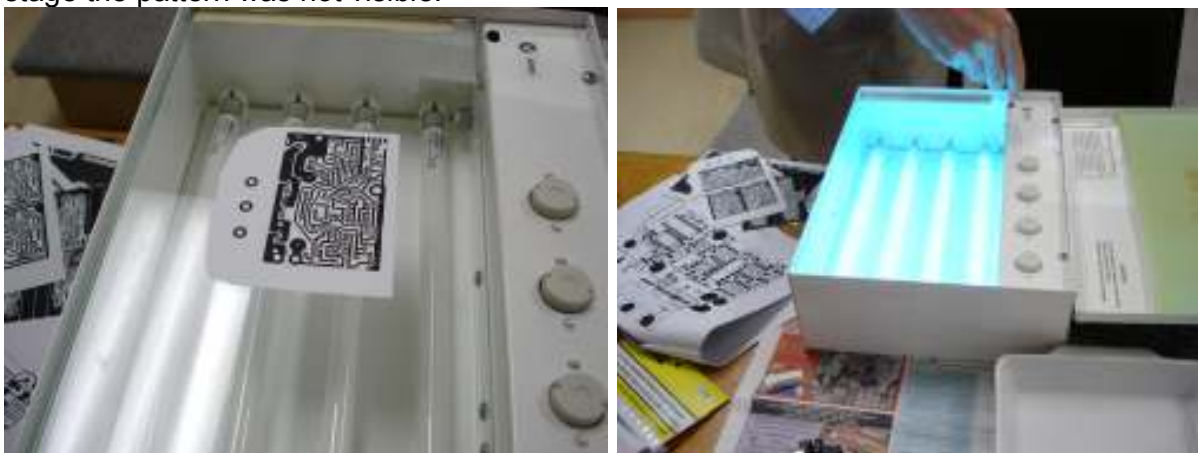
Left photo shows PCB layout ready for sensitized PCB. Right – do not do this at home!
