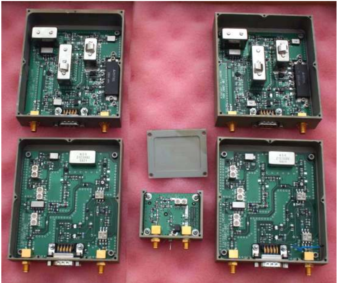
KiwiSAT Linear Transponders complete with preamp Mode US (Transmit 70 cm, receive on 2 m)
