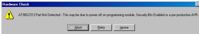
Fig. 6.4 No communications with device to be programmed
