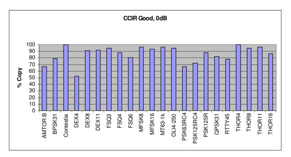
It was pleasing to see that the FSQ modes performed adequately, and although not perfect, they hold up well. They have (at 0dB SNR) a good sensitivity margin, but not enough to survive the deepest fades. The multi-path and Doppler are relatively benign in this test.
