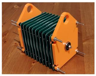
A low-cost, high-voltage butterfly variable capacitor for a magnetic loop antenna: a project which has stalled due to complexity!
