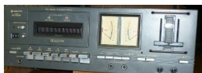
Sanyo tape deck With VDU meters Belt slips
