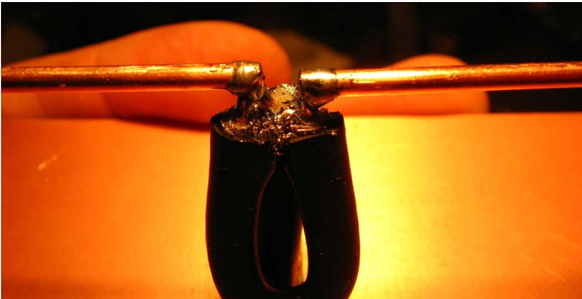
Balun and feeder soldered to radiation dipole
