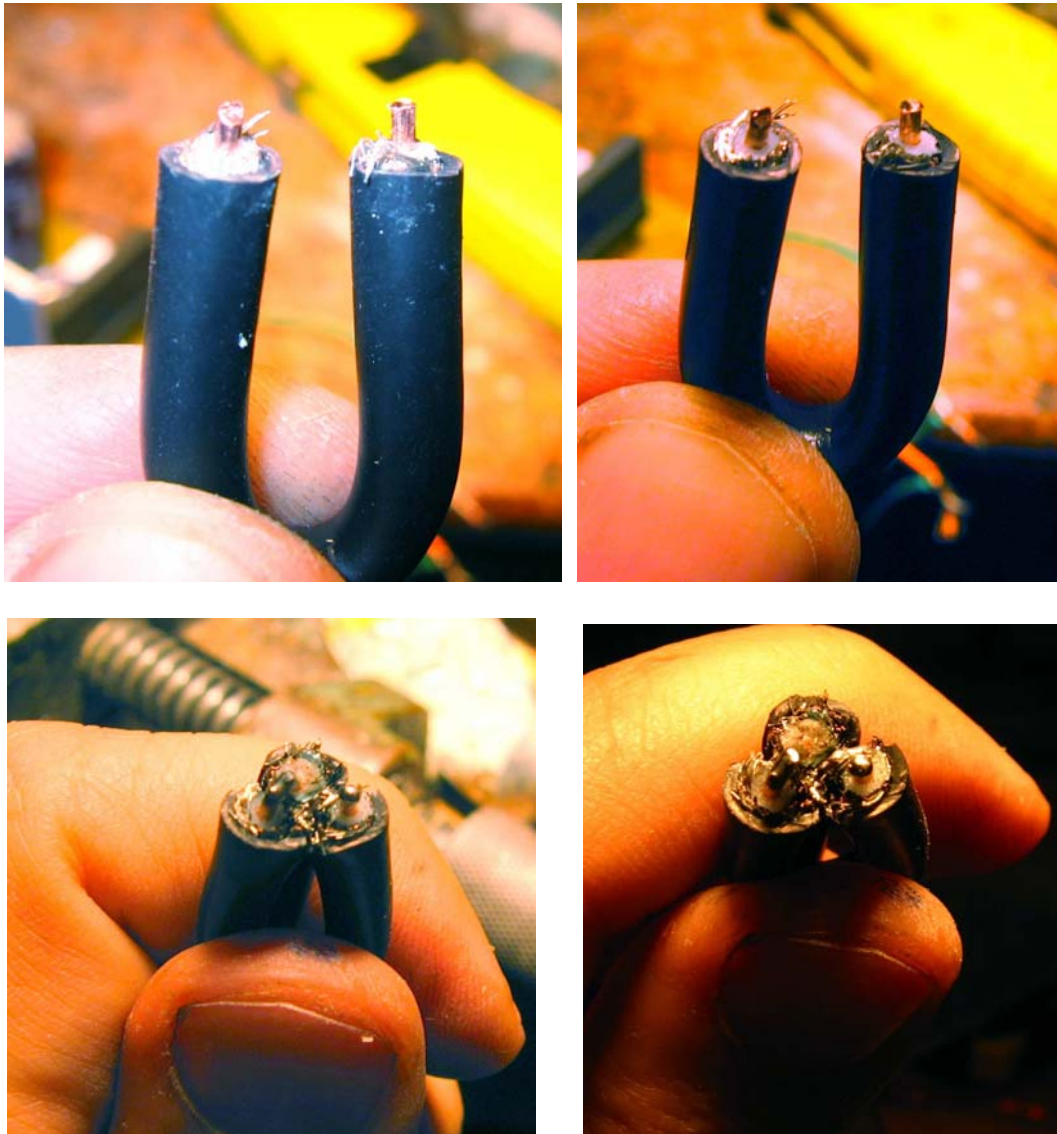
Preparation and soldering of the halfwave balun and coaxial cable
