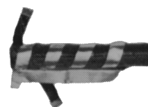
Line Transformer on Ferrite (Figure 30)
